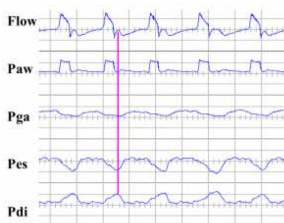
Figure 31: Cycling off - premature opening of exhalation valve
