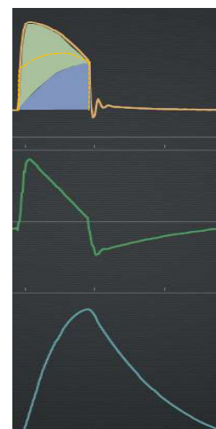
Increased Resistive Load
