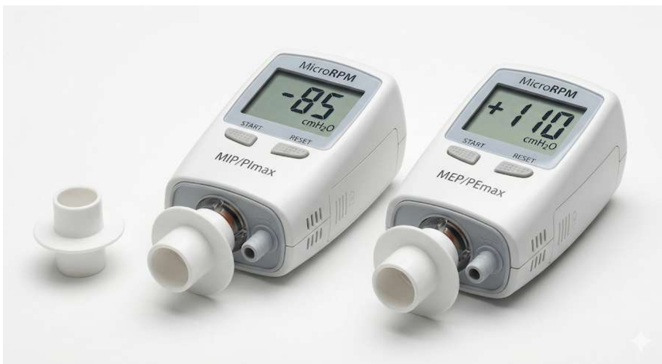
Figure 5D: MIP (left) and MEP (right) manometer schematic diagrams. MIP measured from RV (optimal diaphragm length); MEP from TLC (optimal expiratory muscle length). Report best of \geq 3 efforts within 20 cmH 2 O.
